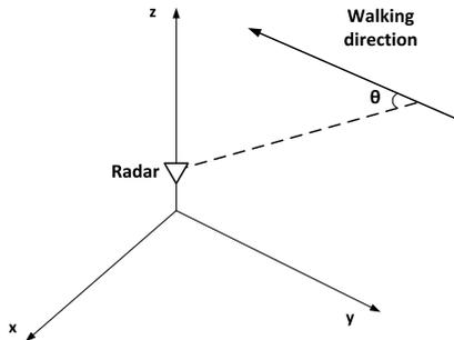
Fig. 10. Illustration of Doppler angle.
