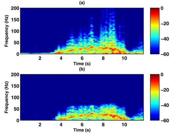
Fig. 3. Spectrogram of a typical series of radar data containing a human walk. (a) Before bandpass filtering; (b) After bandpass filtering. Note that the  $x$  and  $y$  axes have been converted to the continuous time and frequency domains.
