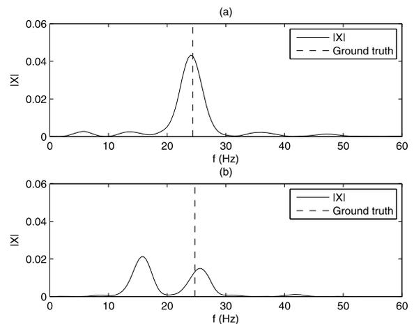
Fig. 7. Robustness analysis of STFT method. (a) Spectrum of the 61st segment (6.25 s). (b) Spectrum of the 72nd segment (7.40 s).
