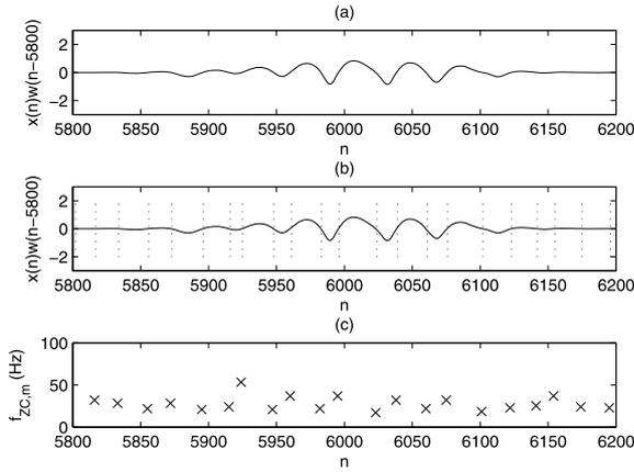
Fig. 4. Illustration of the STZC method. (a) A windowed radar data segment from the first processing step. (b) The radar data segment with zero-crossing points identified by  $n_l$  in the second processing step. (c) The individual zero-crossing frequency estimates from the second step.
