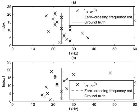
Fig. 8. Robustness analysis of STZC method. (a) Zero-crossing frequency estimates of the 61st segment (6.25 s). (b) Zero-crossing frequency estimates of the 72nd segment (7.40 s).
