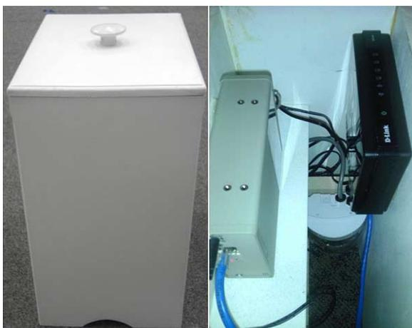
Fig. 1. The radar system. The figure on the left is the wooden box which contains the radar, data logger and the wireless router. The figure on the right shows their deployment inside the box. They are the data logger, Doppler radar and wireless router from left to right.
