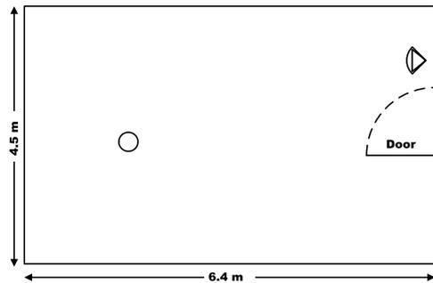
Fig. 11. Layout of the residence experiment of subject #1. The sector and triangle represent the Kinect and radar respectively which are at the same horizontal position. The Kinect is 2.7 m while radar 0.15 m above the ground. The circle represents the subject who generates daily walk behaviors. The locations of the radars and Kinects in the residences of other subjects may be different.
