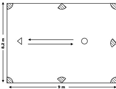
Fig. 5. Layout of the laboratory experiment. The shadowed sectors are the Vicon sensors whose heights are 3 m. The circle represents a male human with height 1.75 m, and the triangle represents the Doppler radar that is 0.15 m above the floor.
