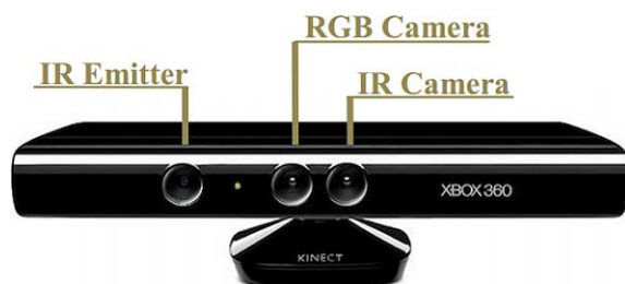
Fig. 1. The Microsoft Kinect sensor with the individual sensors labeled.
