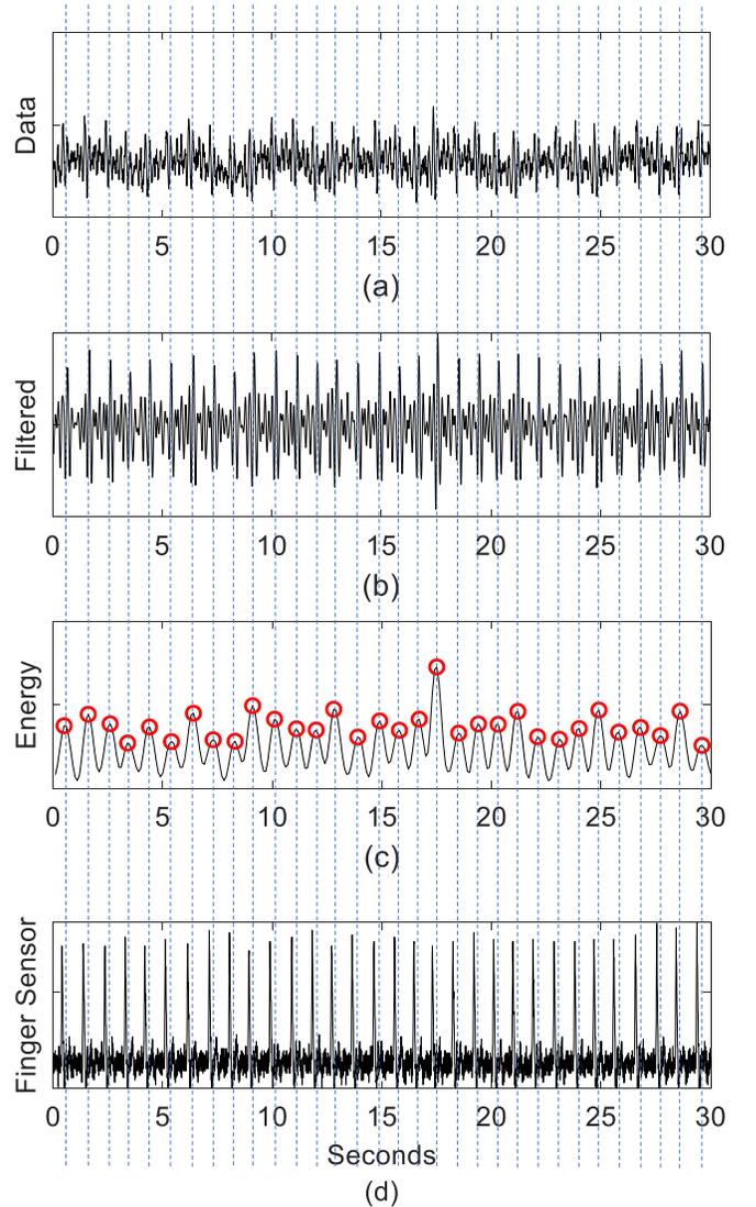
Fig. 2. (a) The 30 seconds signal obtained from hydraulic bed sensor, (b) filtered signal of (a), (c) the energy profile  $E(n)$  where the BPS feature values are the values of the local peaks indicated by circles, (d) the corresponding signal from finger pressure sensor.
