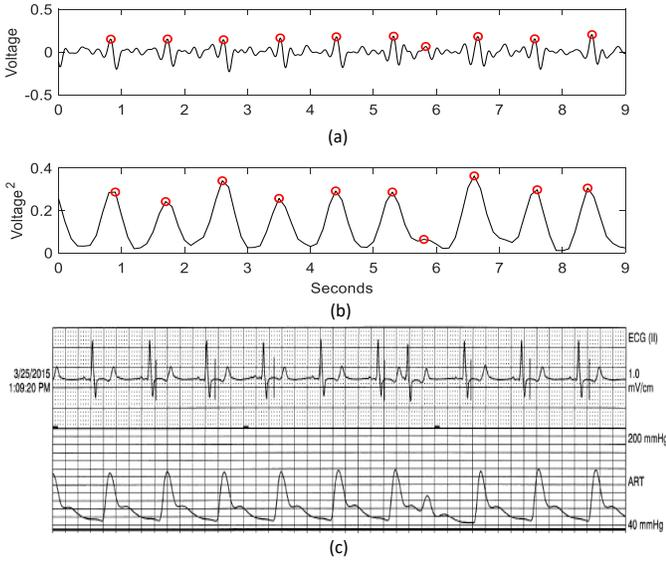
Fig. 3. (a) Pre-processed data from the hydraulic bed sensor, (b) Short-term energy profile of (a), (c) ECG and ART signals.
