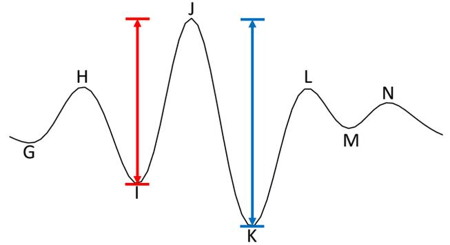
Fig. 4. The illustration of the features extracted from BCG signal to estimate the relative blood pressure.
