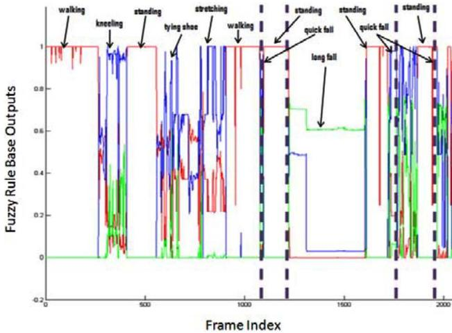
Fig. 10. Approximately 11 min of video analysis, 2042 frames total. A total of four different falls occurred during this time period. The *upright* membership is shown in red, *in-between* membership is shown in blue, and *on-the-ground* is shown in green. Dashed vertical purple lines are the manually inserted moments where a fall occurred.
