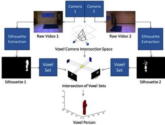
Fig. 2. Voxel person construction. Cameras capture the raw video from different viewpoints, silhouette extraction is performed for each camera, voxel sets are constructed from the silhouettes for each camera, and the voxel sets are intersected to compute voxel person.
