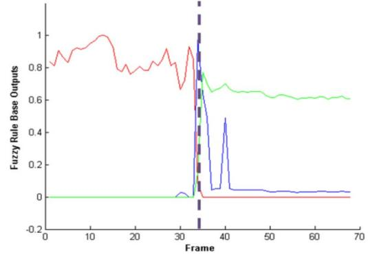
Fig. 7. Fuzzy inference outputs plotted for a voxel person fall. The  $x$ -axis is time, measured in frames, and the  $y$ -axis is the fuzzy inference outputs. The red curve is *upright*, the blue curve is *in-between*, the green curve is *on-the-ground*, and the dashed purple vertical line is where the human indicated a fall occurred. The camera capture rate was 3 fps, so the upper plot is approximately 23 s of activity.
