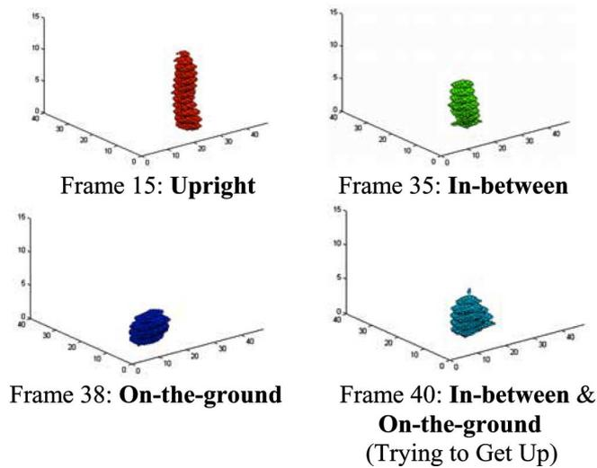
Fig. 8. Color coding of voxel person according to the defuzzified output values. Voxel person's color is a blend of the fuzzy rule system outputs. The *upright* state determines the amount of red, *in-between* is green, and *on-the-ground* adds blue.
